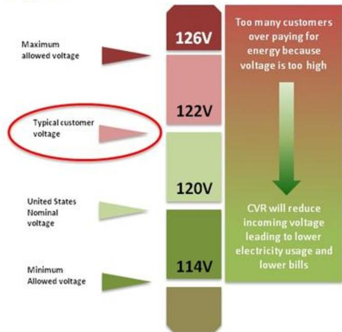
Lacking real-time operating information at the meter, utilities generally deliver energy at a conservative 120V to account for distribution line losses that could cause the voltage delivered
